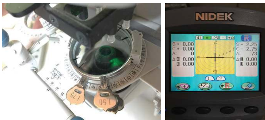
Figure 52: Using a trial frame and lensmeter to calculate a crossed cylinder resultant prescription
